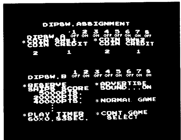
Self-Test - Dip Switch Assignment
